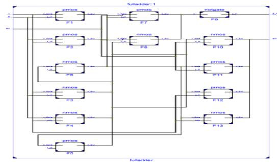
Fig(8).Full Adder RTL Circuit diagram
