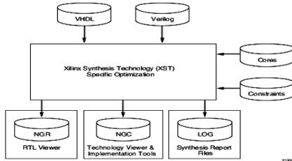
Fig (5): Synthesis tool in Xilinx environment
