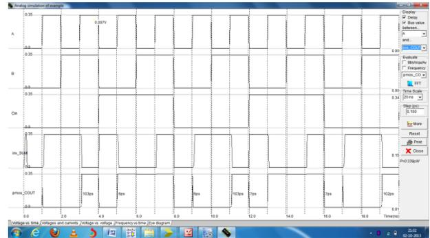
Fig (4): Simulation Results of 14 CMOS Full Adder top module in Micro wind
