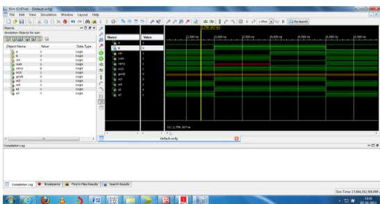
Fig(7).Full Adder Xilinx simulation result
