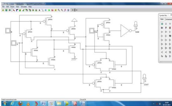
Figure (3) 14 MOS Transistor 1 bit-CMOS Full Adder circuit.
