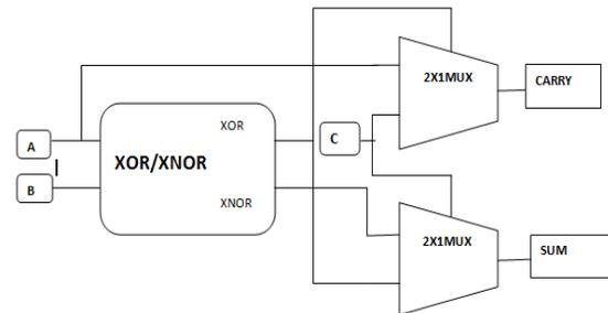
Figure (1) 14 Transistor 1 bit Full Adder Block Diagram
